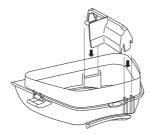
7. Fit the seal onto the rim of the water chamber base. Press along the edge to ensure that the seal is fitted properly.
